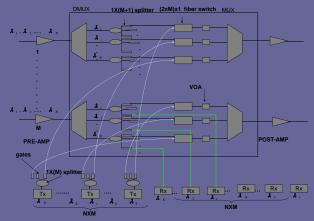
Node design for fixed Txs/Rxs. The number of Txs/Rxs allowed equals the number of wavelengths times the degree of node (i.e., NXM).
