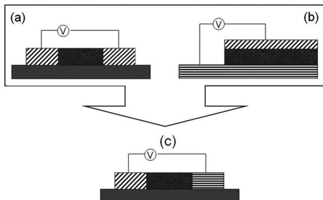
**Figure 1.** Structural models of a coplanar photoconductor with two symmetrical electrodes (a), a sandwich photodiode with two asymmetrical electrodes (b; one is transparent), and a coplanar photodetector with two asymmetrical electrodes (c).
