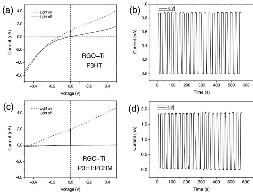
**Figure 3.** a)  $I$ - $V$  characteristics of the AGTE-based photodetector with P3HT as the photosensitive material. b) The on/off characteristics of the P3HT photodetector at 0 V bias. c)  $I$ - $V$  characteristics of the AGTE-based photodetector with the blend P3HT:PCBM as the photosensitive material. d) The on/off characteristics of the P3HT:PCBM photodetector at 0 V bias.
