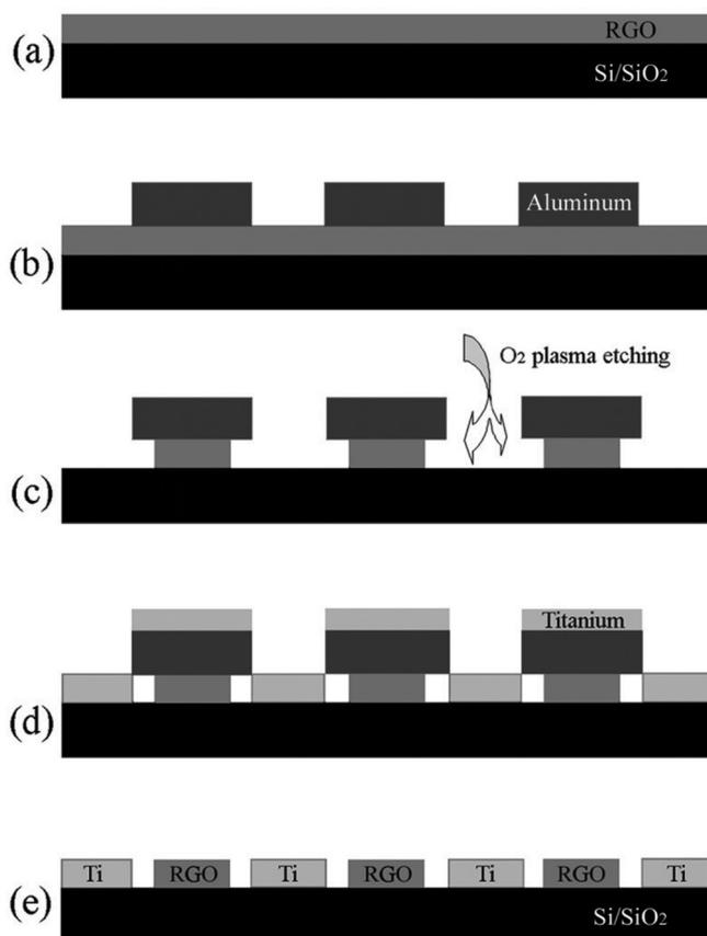
**Scheme 1.** Schematic illustration of the fabrication process of AGTEs. a) A graphene film was produced by thermal reduction of a GO film. b) Patterned aluminum was evaporated to serve as a sacrificial mask. c) An undercut along the edges of the aluminum patterns was formed by long-time oxygen plasma etching of the graphene film. d) Titanium electrodes were evaporated directly on the etched film. e) Patterned AGTEs were obtained by washing away the sacrificial aluminum layer.
