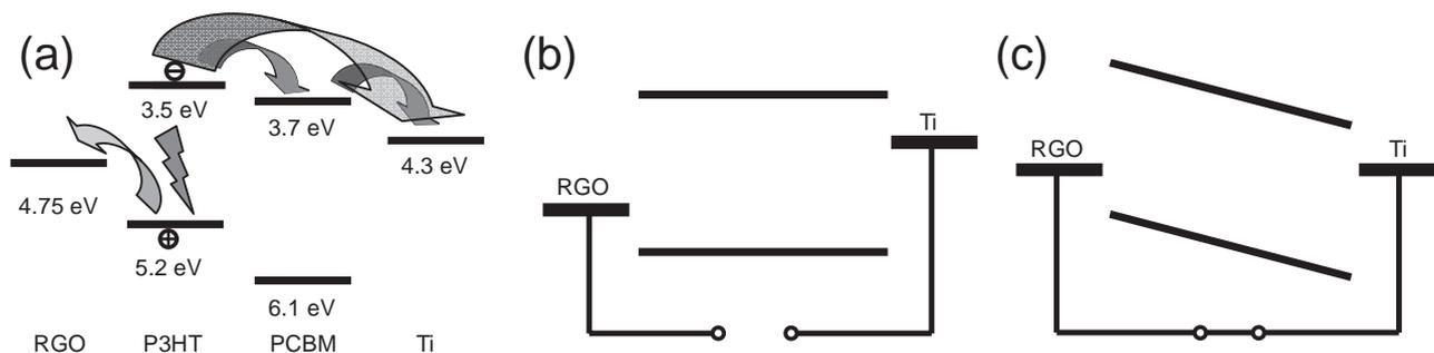
**Figure 5.** a) A schematic representation of charge transfer and transport as an energy level diagram. b,c) Simplified principles of device function for organic semiconducting layers between two metallic electrodes: open-circuit (flat-band) condition (b) and short-circuit condition (c).
