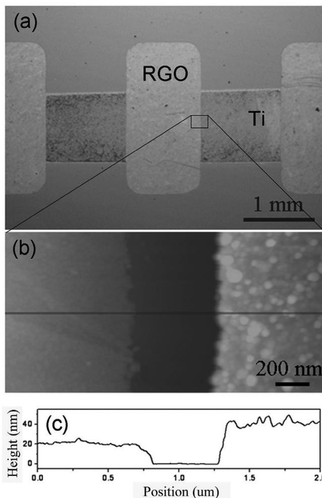
**Figure 2.** a) OM image of AGTEs; white rectangles are RGO and darker squares are Ti. b) AFM image of the edge of the RGO-Ti electrodes, indicating a channel length of ca. 500 nm. c) Height profile along the line in (b), showing a narrow channel etched down to the underlying  $\text{SiO}_2/\text{Si}$  substrate.
