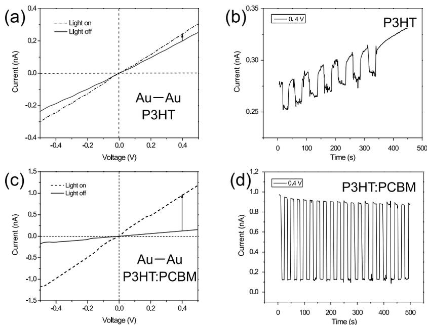
**Figure 4.** a)  $I$ - $V$  characteristics of the symmetrical gold electrode-based photodetector with P3HT as the photosensitive material. b) The on/off characteristics of the P3HT photodetector at 0.4 V. c)  $I$ - $V$  characteristics of the symmetrical gold electrode-based photodetector with the P3HT:PCBM blend as photosensitive material. d) The on/off characteristics of the P3HT:PCBM photodetector at 0.4 V.
